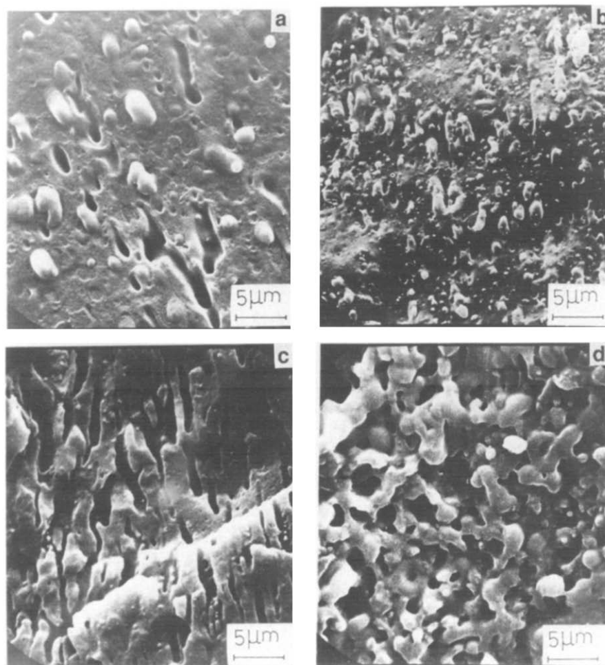
Figure 2 SEM micrographs of the directly quenched SEBS/poly(ether ester) blends with the compositions 20/80 (a, c) and 50/50 (b, d). (a, b) Fracture surfaces; (c, d) fracture surfaces of the extracted blends
